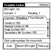
These are the self-diagnostic tests that the computer does to make sure the equipment is working. Tests are listed by name, then their status. In the example above, the Catalyst self-test has been completed (YES), the Heated Catalyst test is not supported in this car (NA – means this car doesn't have one), and the Evap System test has not been completed (NO).
